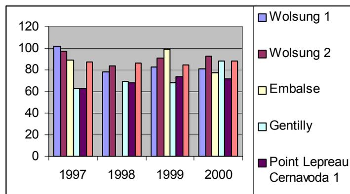
FIG. 3. CANDU 6 NPP Gross Capacity Factor
